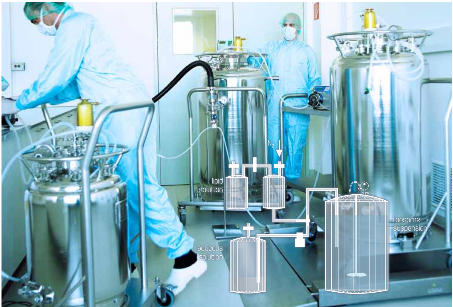
LIPOSOMAL FORMULATION IN THE cGMP PRODUCTION SCALE: 250 L IN 1.5 HOUR
